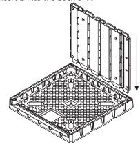
3. Insert  $\underline{\mathbf{C}}$  into  $\underline{\mathbf{A}}$  (one at a time) making sure corner joints intersect
