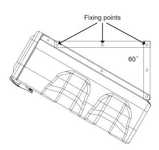
Use the pre-drilled holes on the back of the box when attaching the mounting brackets.
