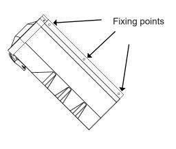
The extinguisher must not rest on top of the tension strap.
